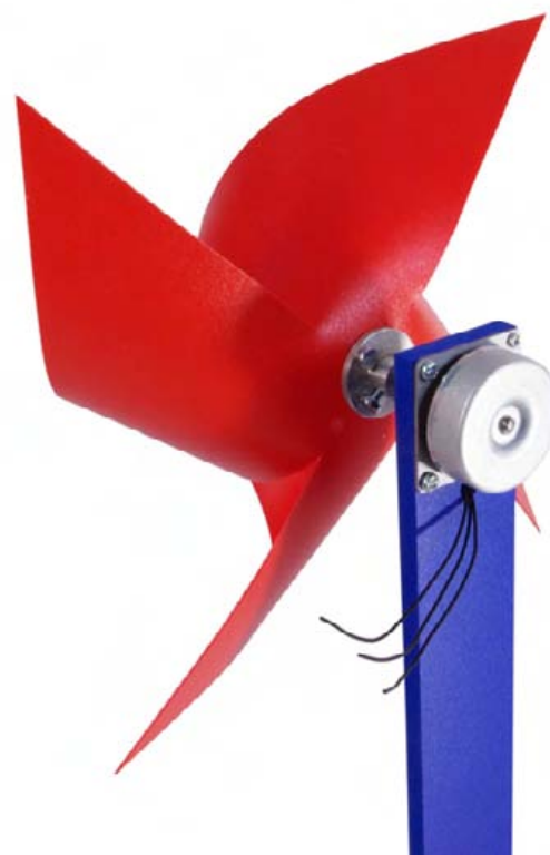
Example of a different assembly of this detailed in this folder : here the electric part remains fixed. The DEL can then be fixed on the support or deported further to simulate a building power supply.
